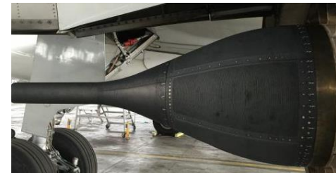
Lined plug prototype (1 st generation)
